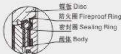
软密封防火结构 (图d) Soft Seal Fireproof Structure (fig.d)
